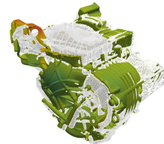
3D FEA Electric Drive Unit incl. gears
